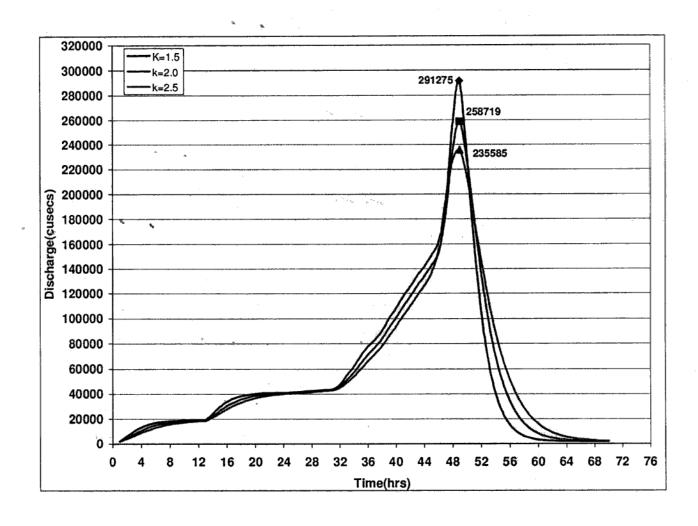
Fig 5: PMF hydrograph computed from the 3 different UH ordinates
