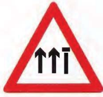
Lane Closed (Three Lane Carriageway)
