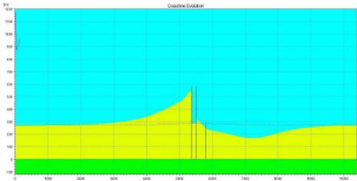
Fig.6(A) Model output in terms of shoreline after 10 years of simulation
